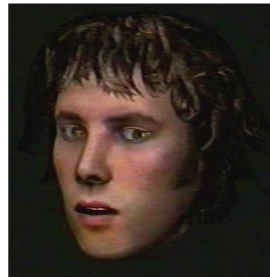
Figure 4 - Geppetto 60 fps real-time model using bones for hair deformation and vertex morphing and blending for facial expressions
